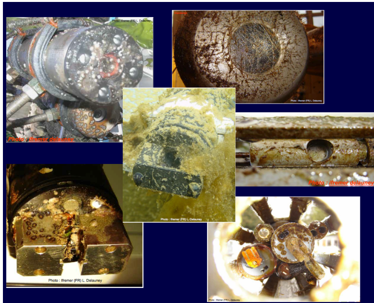
FIGURE 5 FOULING ON THE SENSORS IS THE MAIN CONSTRAINT FOR IN SITU OCEAN AUTONOMOUS MEASUREMENTS
